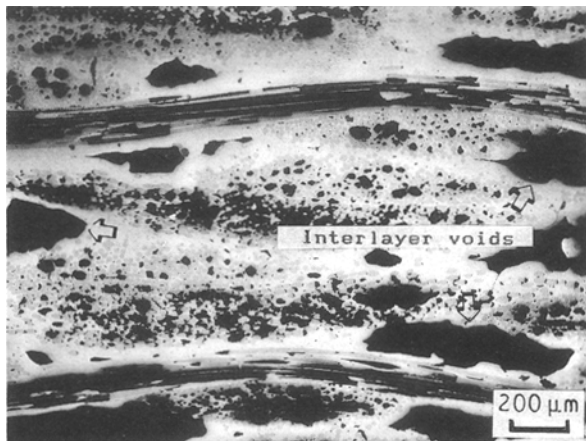
Figure 3 The optical micrograph of the as-received 2-D woven laminate Nicalon/SiC composite.
