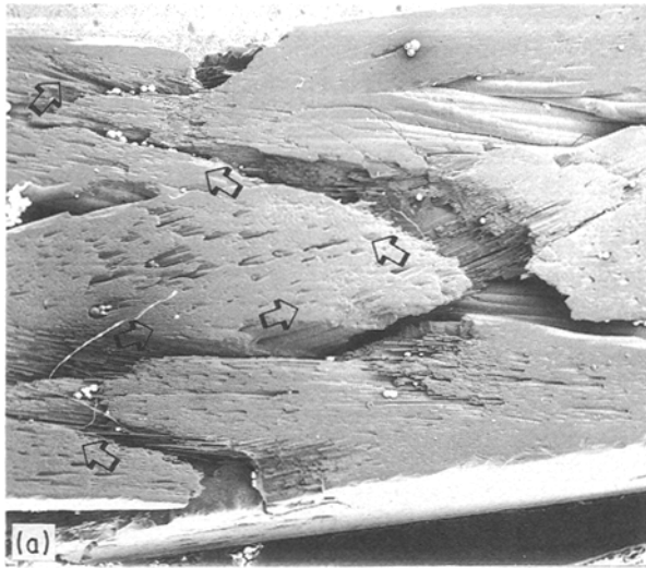
Figure 7 The crack propagation pattern of the as-processed (a) 3-D braided, (b) 2-D woven laminate Nicalon/SiC composite.
